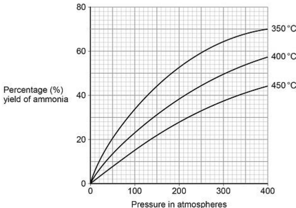
A temperature of 450 °C and a pressure of 200 atmospheres are used in the Haber process.
